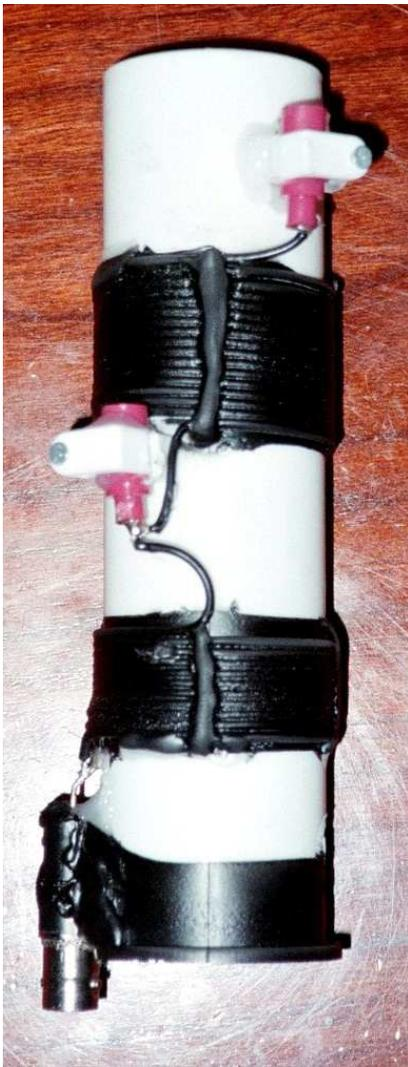
The picture to the left shows the coil or main antenna part. This was my prototype coil and I still use it today as it works great! The coil form is nothing more than a 6" plumbing sink extension I bought at Home Depot for around \$2.00 or less. The O.D. of the coil form is 1-7/16 inches. This is what the coils are wound on.
